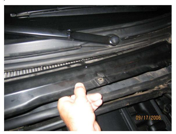
Take note of how the filter fits in the assembly, and then remove the filter.
