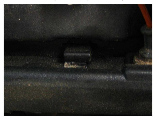
Once the coil wires are moved, you can pull up gently on the wires underneath. These are just held by some simple U-clips. Only the one held by my finger in the photo is tricky, just lift the tab and pull the wires out from the side (this is right above one of the oxygen sensors, so don't bust the wire off the top of the sensor). As a note, I did not disconnect any wires, I just moved them out of the way. These wires I twist-tied to the heavy battery cable running above the engine.
