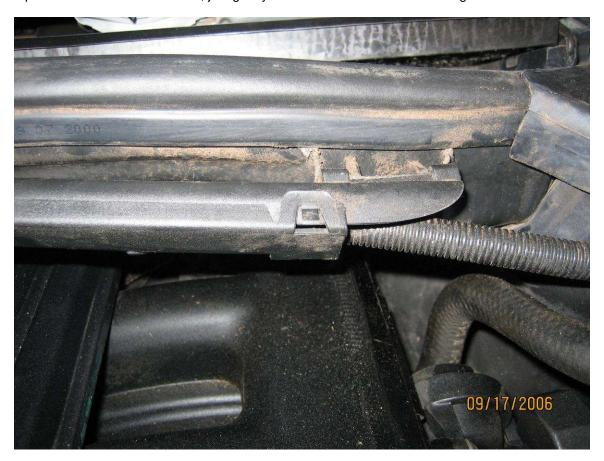
Remove the four TORX bolts using a T30 bit. The screws are about an inch long, so keep twisting until they are all the way out. Lifting on the front of the filter tray, gently work it out of its spot. This part is done.
