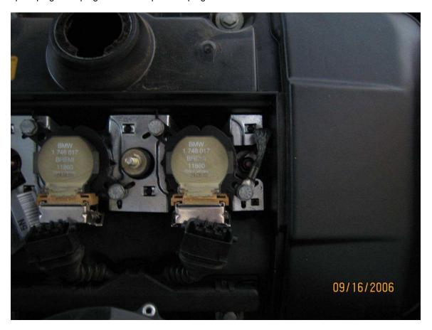
Everything is out. Soon we will remove the entire electrical assembly holding the coil wires.
