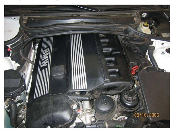
The entire cabin filter assembly should be removed for easy access to the engine. This is very easy, and only takes about 15 minutes.
