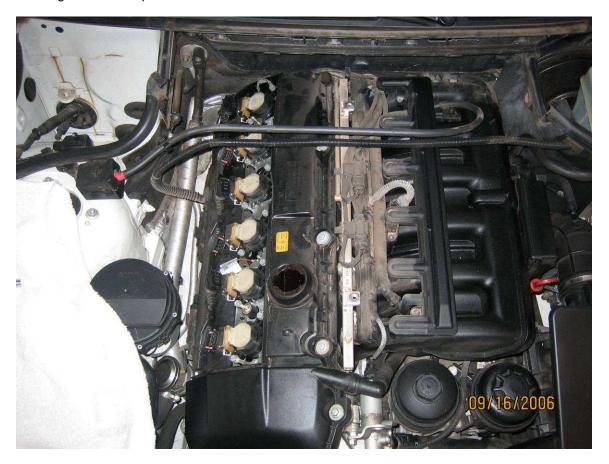
I forgot to take this photo, but Tim P.'s spark plug replacement instructions do a good example of showing how to undo the clip holding the coil wire in place. I did not need to use a screwdriver, but you might. The metal clip just slides up, and you can easily pull the coil plug out from the side. Just be very gentle (a common theme).
