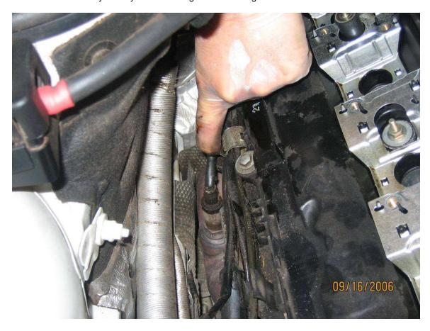
No you can finally start removing the valve cover hold down bolts. All of them are 10mm. This photo shows one of the center ones coming out. Every bolt has a metal washer, then a rubber gasket. Replace the gaskets on your install, mine looked pretty used (see next photo). Once all the bolts are removed, pull the valve cover up to remove it. I had to gently pry mine in a few places.
