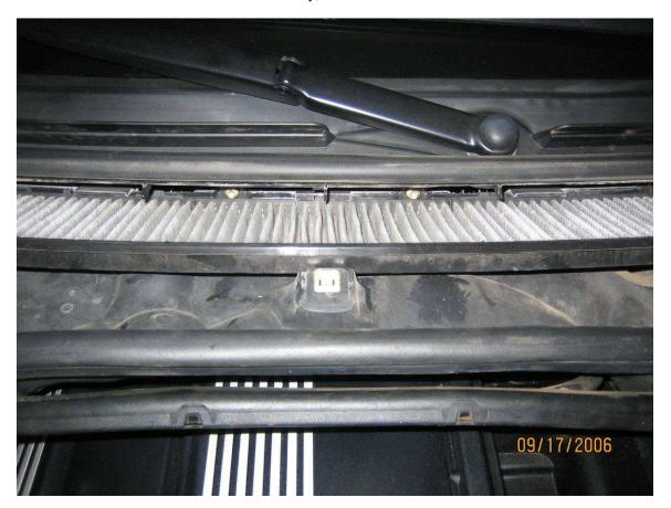
The wires running in front of the cabin filter assembly are covered by a flat lid. Each side of the lid has simple snap connectors like the one shown. Just gently lift the tabs while working the lid off. Once the top side connectors are undone, just gently roll the lid off the channel holding the wires.
