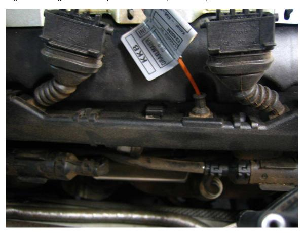
The clip as described in the prior step. When reinstalling the assembly, just make sure it is lined up and press it down. It will click back in place. This was pretty slick, BMW did this right.
