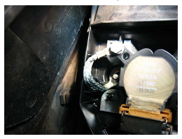
Remove this wire with also; it too has an 8mm nut. Once it is off, you will notice that there are four 10mm bolts now exposed on the valve cover top. One was covered by this wire, two were covered by the ground straps. All four of these will need to be removed, they look like nuts, but they are really 10mm bolts.
