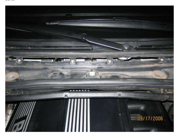
Using a flat head screwdriver, gently pry off the engine cover bolt caps. Using a 10mm socket, remove the bolts and nuts. The right side engine cover should be pulled to the left as it is removed (remember to reverse this procedure when putting everything back together).
